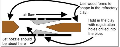
\*The lenght of the tube is only an indication. For proper lenght, make sure that the jet is slightly downstream from the air intake holes. If the lenght is well ajusted, the clay venturi might not be needed.
